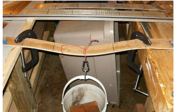
Testing how much weight a piece of wood can support before breaking
