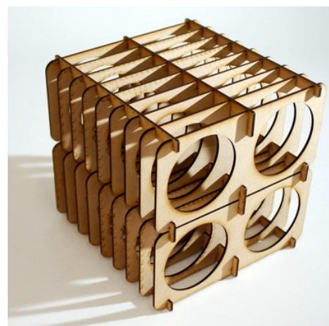
2D flat Laser cut Plywood that can be assembled to represent 3D objects
