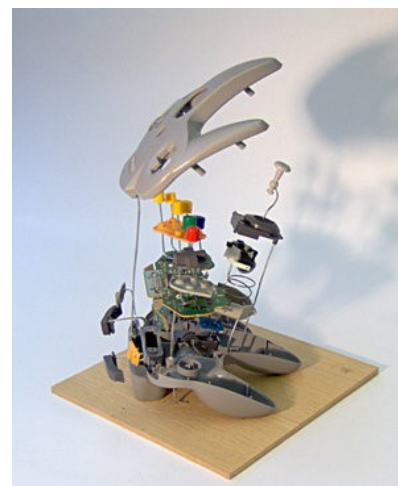
Computer mouse taken apart to understand how it works
